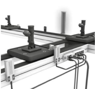
RFID supports process control: Are the parts being brought to the right production stage at the right time?
